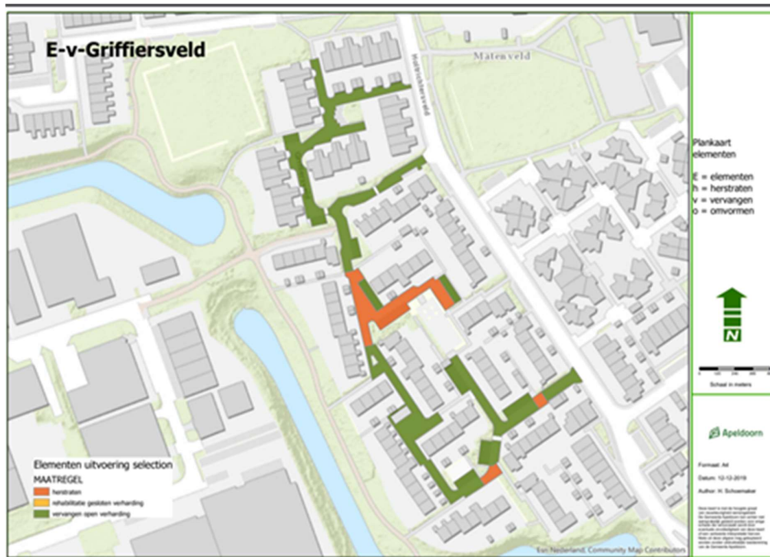
Figure 14. New plan for the renovation of Griffiersveld. The green parts are only renovated lightly by changing the pavement, but the red parts will be completely renewed with new drainage system etc.
